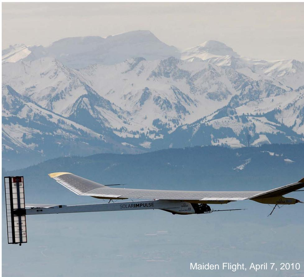
63 m wingspan, 12,000 solar cells, zero kerosene
